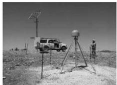
**Figure 2** A GPS receiver and antenna permanently installed for precise monitoring motion of the earth's crust. Site Benares in California in the US. Photo taken from aircraft at <http://www.cnr.gov>
