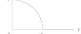
Figure 1. Spontaneous magnetisation: the magnetisation m(T) is a function of the temperature T . For a typical configuration of the spins, m(T) is the difference between the number of spins pointing up and the number of spins pointing down, divided by the total number of spins. The temperature T_c is the temperature at which there is a critical transition, T_c below which the system exhibits a collective behaviour in that a majority of them point in the same direction (either a majority up or a majority down ). An ordering configuration with the opposite magnetisation -m(T) is equally likely.
