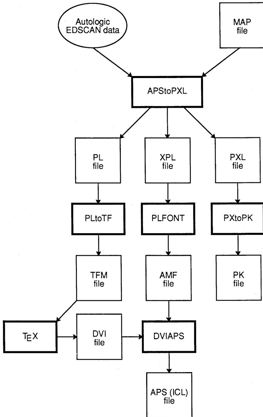
Figure 1: Overview of creation of Autologic fonts for use with TeX
