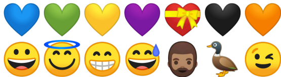
Figure 3: Random Unicode emojis using Noto Color Emoji font which embeds bitmap PNGs instead of outline glyphs. (Grayscaled in the print version.)
