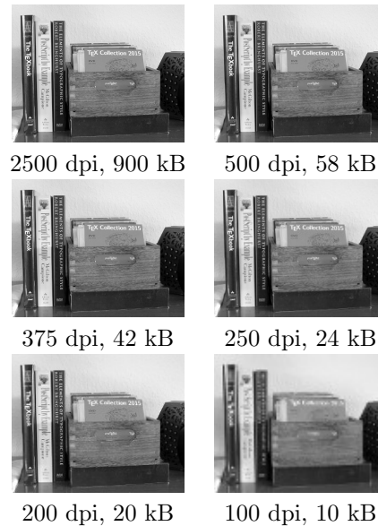
Figure 1: The same photograph in several resolutions. See for yourself where quality degradation becomes perceptible.
